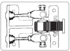
3.1 Pedal Depressed Balance Bar not at an angle (Correct)
