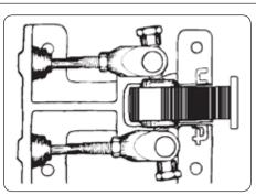
3.2 Pedal Depressed Balance Bar at an angle (Incorrect)
